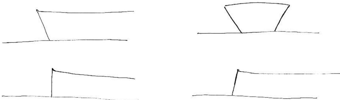
This transom view in the body plan does not tell us if there is a rake or not. Each of the three profiles could be it. Each has different dimensions (and diagonals are longer than the vertical line)
