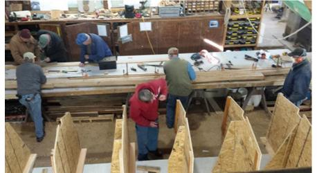
By building a variety of boats from scratch we've been able to expand our programming to encompass more than the wooden construction of the vessel to include sail making, metal casting, foundry work, diesel mechanics and the installation of systems.
